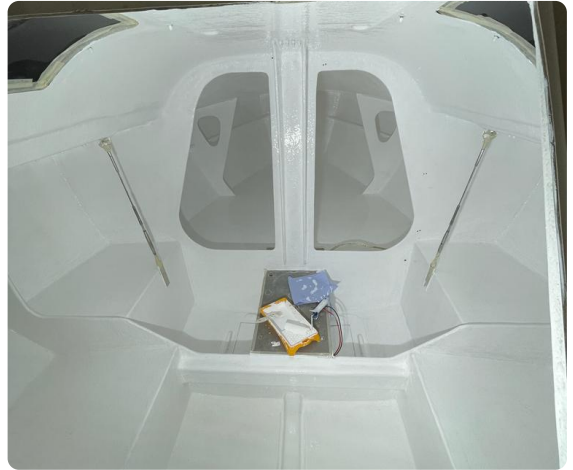
Interior stripped, sanded and repainted during the electrical rebuild
